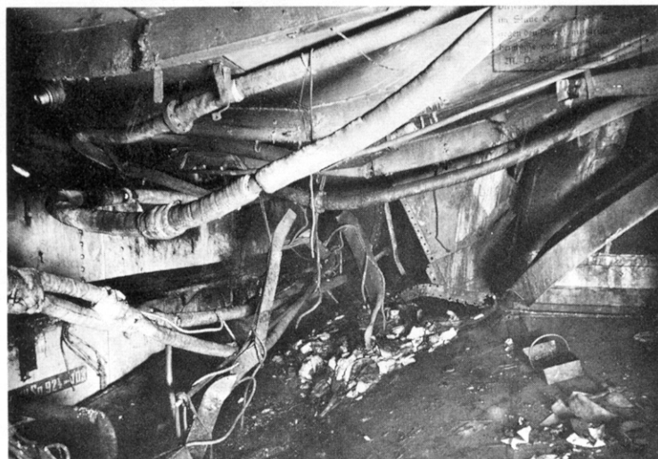
SMS König hit under deck. The sign in the picture indicates a ventilator extending from frame 92½ to 103, an area which housed ammunition and secondary steering positions. Jutland 1916. (Bundesarchiv)
