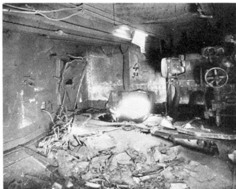
A hit by a large calibre shell at Frame 93 on König, suffered at Jutland. The gun in the picture is the foremost port 5.9in casemate gun. (Bundesarchiv)
