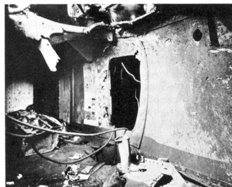
SMS König hit under deck. The sign in the picture indicates a ventilator extending from frame 92½ to 103, an area which housed ammunition and secondary steering positions. Jutland 1916. (Bundesarchiv)
